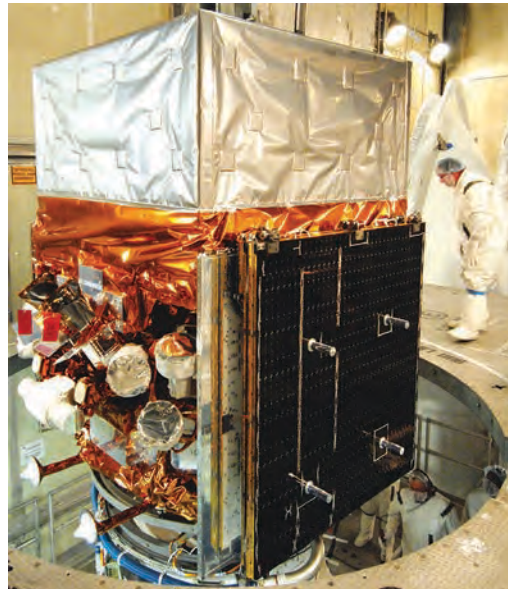
The Fermi spacecraft shortly before launch. The solar panels are folded at the sides. The GBM detector modules and the telemetry antennas can be seen on the left side.
