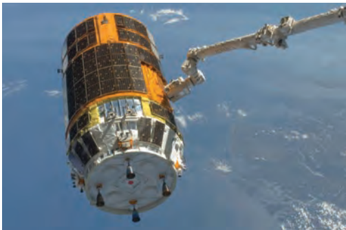
The International Space Station's Canadarm2 unberths the unpiloted JAXA HTV-3, filled with trash and unneeded items, in preparation for its release from the station.
