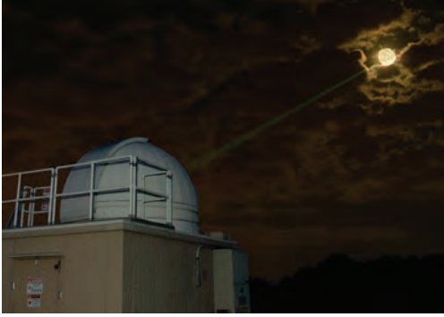
NASA's Next-Generation Satellite Laser Ranging (NGSLR) system, located at the Goddard Geophysical and Astronomical Observatory in Greenbelt, Maryland, is shown ranging to the Lunar Reconnaissance Orbiter orbiting the Moon. This process provides the information needed to model the onboard clock drift and allows high-precision orbit determination.
