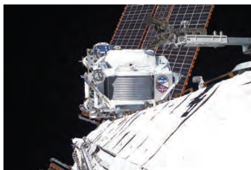
The AMS-02 after installation on the International Space Station's (ISS) S3 Upper Inboard Payload Attach Site on the S3 Truss segment. The AMS-02 will remain active for the duration of the ISS Program.
