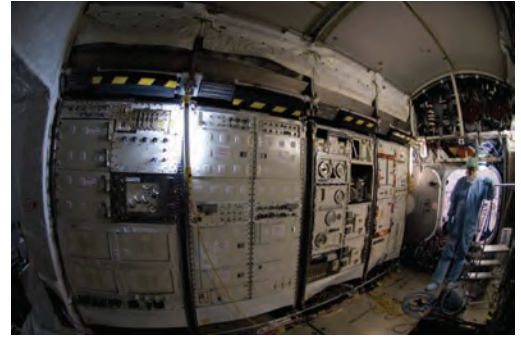
An interior view of the European Columbus Laboratory at the Space Station Processing Facility at NASA's Kennedy Space Center in Florida as the module is prepared for flight to the International Space Station: European Drawer Rack (left), European Physiology Modules Facility (center), Biolab and Fluid Science Lab in the launch configuration (right). (Credit: European Space Agency/S. Corvaja)
