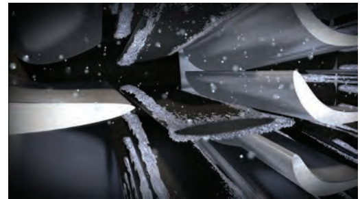
Polar opposites attract in the puzzling case of ice crystal engine icing, where the frozen crystals can be ingested into the core of a jet engine.
