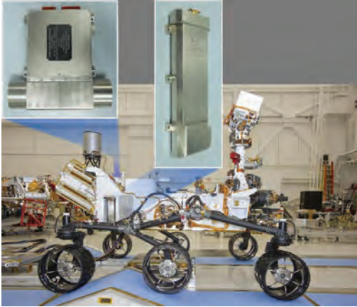
This image of NASA's Curiosity rover shows the location of the two components of the Dynamic Albedo of Neutrons instrument. The neutron generator is mounted on the right hip (visible in this view), and the detectors are on the opposite hip. (Credit: NASA/Jet Propulsion Laboratory–Caltech)
