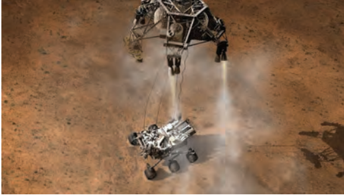
This artist's concept depicts the moment immediately after NASA's Curiosity rover, lowered via a unique sky-crane system, touched down onto the Martian surface. After the spacecraft detected the touchdown, pyrotechnic cutters severed the connections between the rover and the spacecraft's descent stage, which then flew away, coming back to the surface a safe distance away. (Credit: NASA/Jet Propulsion Laboratory—Caltech)
