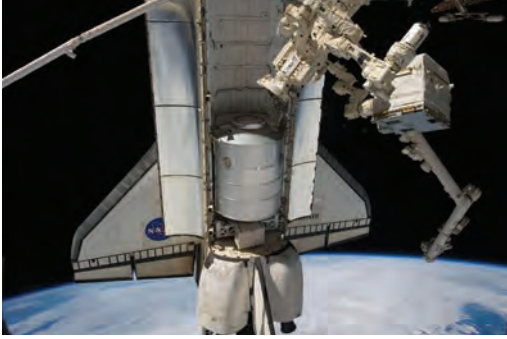
The former Leonardo MPLM arrives via STS-135 at the International Space Station (ISS), where it takes up residence as a permanent ISS module, adopting the new name of Permanent Multipurpose Module (PMM). The PMM adds an additional 2,472 cubic feet of stowage and science activity space to the ISS.
