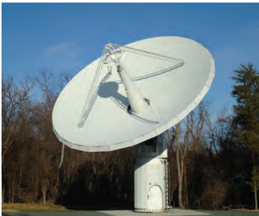
This 12-meter antenna is part of the next-generation geodetic Very Long Baseline Interferometry system at NASA's Goddard Geophysical and Astronomical Observatory in Greenbelt, Maryland. Essential new features include the fast antenna, broadband receiver, and high-rate recording at four settable bands.
