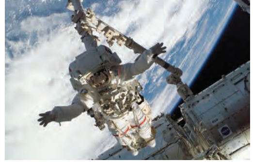
Astronaut Rick Linnehan conducts a spacewalk during the STS-123 mission while anchored to a Canadarm2 mobile foot restraint. During the spacewalk, Linnehan helped install the tool-change-out mechanisms on the Canadian-built Dextre robotic system, the final element of the ISS Mobile Servicing System.
