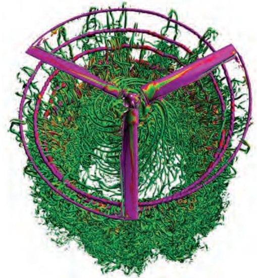
A Navier-Stokes simulation of a V-22 Osprey rotor in hover; magenta indicates high vorticity, and blue indicates low vorticity.
