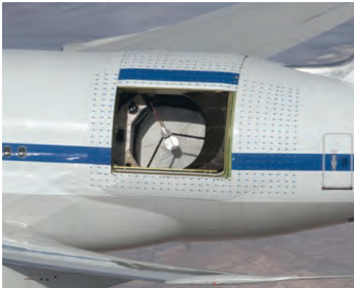
A close-up of the SOFIA telescope in flight.
