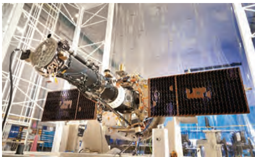
The fully integrated spacecraft and science instrument for NASA's IRIS mission is seen in a clean room at the Lockheed Martin Space Systems facility in Sunnyvale, California. The solar arrays are deployed in the configuration they will assume when in orbit. (Credit: Lockheed Martin)
