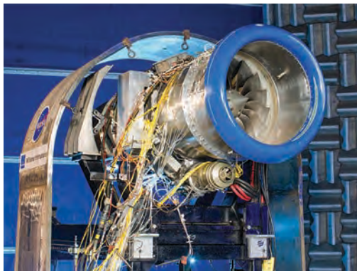
A test rig is assembled at NASA's Glenn Research Center to evaluate the noise reduction of a newly developed metallic foam liner.
