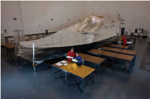
Designed to block solar light and keep the JWST observatory operating at cryogenic temperature, the five-layer sunshield consists of thin membranes made from a polymer-based film and supporting equipment such as spreader bars, booms, cabling, and containment shells.
