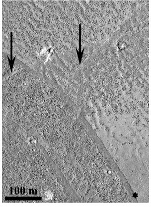
**Figure 1.** Thin, overlapping flows north of the Cerberus Fossae in HiRISE image PSP\_001408\_1900. Traces of buried flow fronts are indicated by arrows, and a star marks the location where a flow front height of <1 m was measured. Two bright-rayed Zunil secondary craters are visible, one between the arrows and the other to the right of the scale bar.
